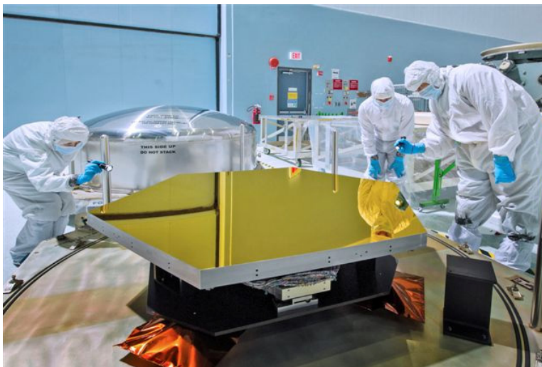
FIGURE 1.9 Technicians and scientists check out one of the James Webb Space Telescope's first two flight mirrors on September 19, 2012, in the clean room at NASA's Goddard Space Flight Center in Greenbelt, Maryland. SOURCE: NASA.
