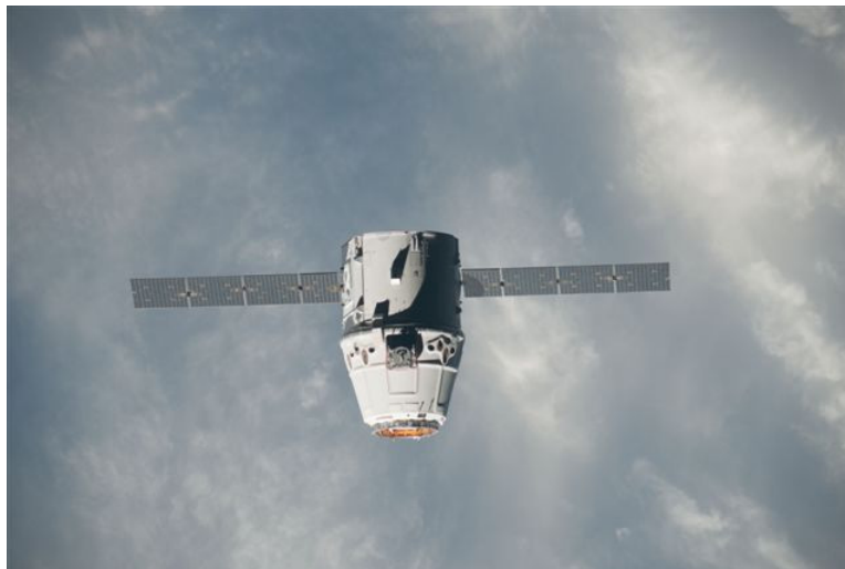
FIGURE 1.12 The SpaceX Dragon commercial cargo craft approaches the International Space Station on May 25, 2012, for grapple and berthing. SOURCE: NASA.
