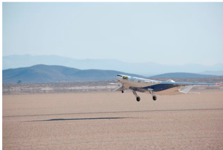
FIGURE 1.10 The NASA X-48C, which is a remotely piloted model of a hybrid wing body aircraft, takes flight for the first time. This aircraft is used for developing new fuel efficiency technologies. SOURCE: NASA/Tony Landis.
