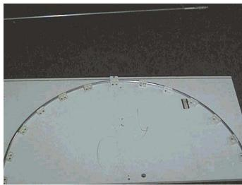
were inserted into this section and screwed firmly in place with 2 zinc screws. At the top, a space between the two sections was left to seperate the top of each half of the loop.
