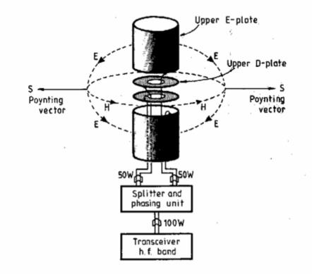
Fig.6. The "barrel-shaped" crossed-field-antenna (CFA).
