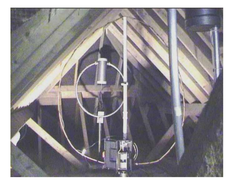
A 'small antenna' is contained inside a sphere of radius  $\lambda/2\pi$
