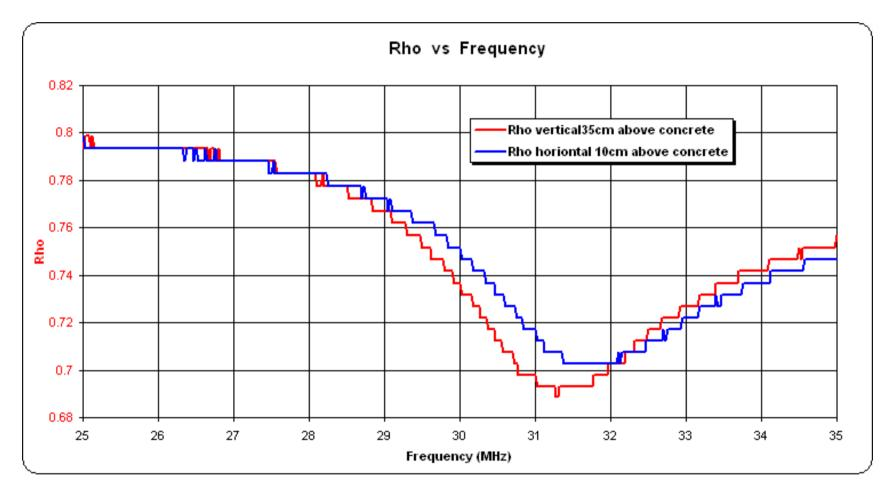
Figure 25: Dry concrete vertical/horizontal comparison showing resonant absorption at about 31MHz using three turn loop with two turns shorted.
