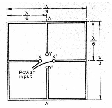
Fig 3. Isolated inputs of the new quad element
