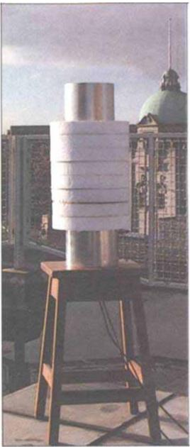
Fig.7. A practical barrel-shaped CFA. The length of this particular structure is 70cm.
