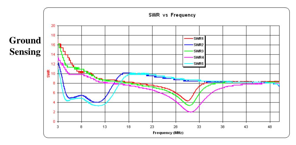
**Figure 24: Two sets of comparisons over wet clay ground.** The lower curves on the left were for a three turn loop. Those curves that are lower on the right were foe a ingle turn with the two turns shorted. SWR 2 and 3 are for the three turn loop vertical and horizontal on the ground respectively. SWR4, 5 and 1 are for the one turn loop vertical and horizontal on the ground and then horizontal and raised 30cm above ground, respectively
