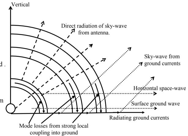
Where does the input power go? How much power couples straight into the ground under a small antenna? Does this propagate under the ground? What is the pattern and polarisation of the antenna when close to ground as compared to free space? How much surface/ground wave is launched, and of what type? Are there two or more surface wave layers. Heuristics can answer all these questions – existing theory and simulations just cannot!
