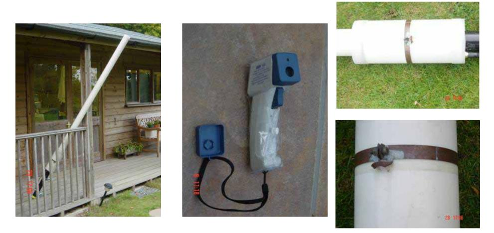
**Arno Venus 160 EH Dipole**: copper 'tuning band' shorted turn temperature increased from 13°C to 25°C using a non-contact thermometer (centre picture) after 15 minutes of 80 watts input to antenna. Rough estimate of no worse than 50% antenna efficiency from this. Needs more refinement.
