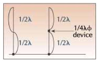
Figure 4. Stacking two half-wavelength radiators normally produces a phase-cancelled signal. (This is the Franklin Antenna)
