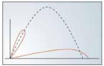
Figure 3. High angel signales cause skywave interference to the groundwave
