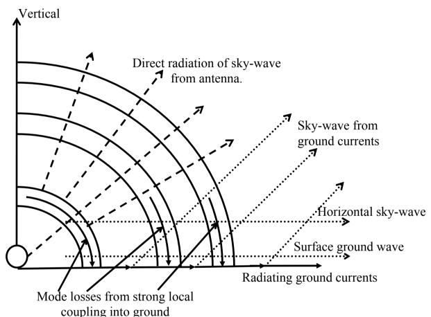
How can we possibly define the efficiency of any small antenna on an absolute basis without knowing all these? Is simulation good enough?
