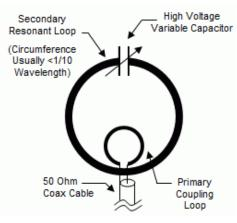
Diagram of a Small Loop Antenna
