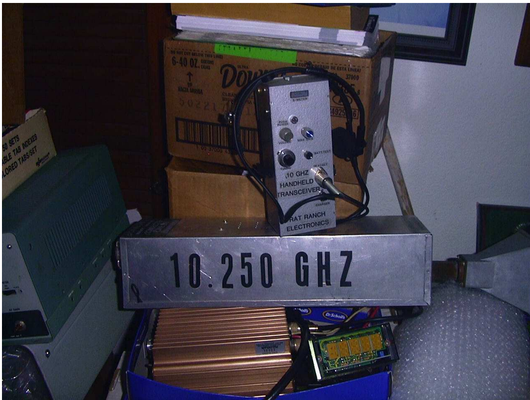
Homebrew 10Ghz Wideband FM sets (Including the one and ONLY 10Ghz Handytalkie!)
