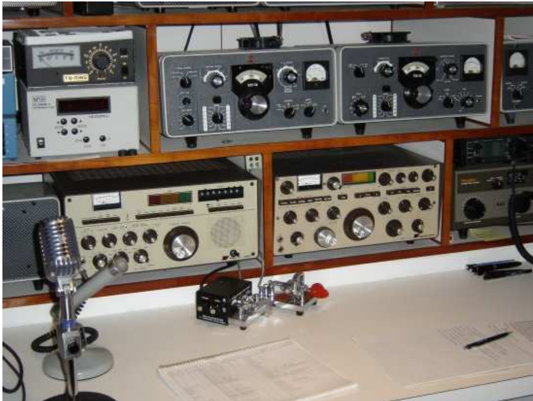
Current configuration: I now am the happy owner of Signal/Ones' two best efforts; the MilSpec 1030 (on the left) and the CX-11A (on the right). The Collins S3 line is on the second shelf. Not shown are the amplifiers; a 30S-1 for the S-line and a Alpha 77Sx/Dx for the Sig/Ones.
